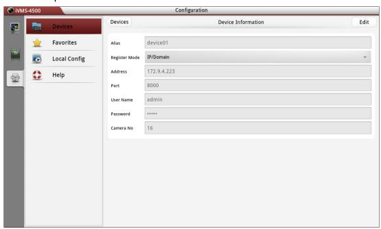
2. Click Edit and then modify the parameters of the device according to actual needs.
