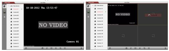
You can drag and move the window to adjust the window sequence. Double-click the live view window to display the camera in 1-division mode and double-click again to restore.
