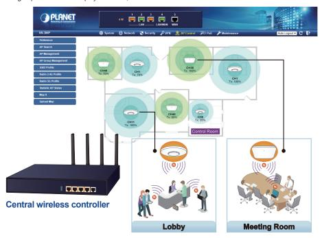
For example, to configure multiple Smart APs of the same model, the VR-300W6A and VR-300PW6A allow clustering them to a managed group for unified management. According to requirements, wireless APs can be flexibly expanded or removed from a wireless AP group at any time. The AP cluster benefits bulk provision and bulk firmware upgrade through single entry point instead of having to configure settings in each of them separately.
