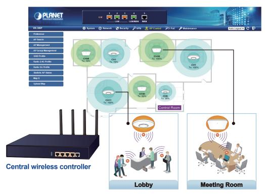
For example, to configure multiple Smart APs of the same model, the VR-300W5 and VR-300PW5 allow clustering them to a managed group for unified management. According to requirements, wireless APs can be flexibly expanded or removed from a wireless AP group at any time. The AP cluster benefits bulk provision and bulk firmware upgrade through single entry point instead of having to configure settings in each of them separately.
