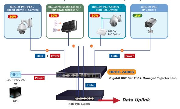
With data and Power over Ethernet from one unit, the HPOE-2400G can reduce power cable deployment and eliminate the need for dedicated electrical outlets on the wall, ceiling or any unreachable place.
