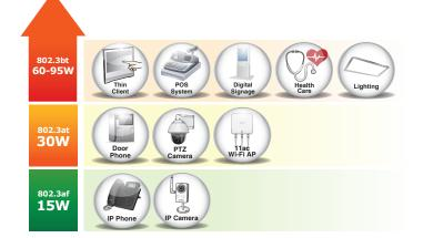
The POE-175-95 delivers the Ethernet digital data with 54V DC power over the twistedpair cables as a 95-watt Power over Ethernet Injector, and the connected ultra Power over Ethernet splitter, the POE-172S, will separate the digital data and the power into three optional outputs (12V/19V/24V DC) with distance up to 100 meters.
