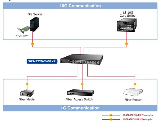
By means of improving the technology of Optical Fiber Ethernet with highly-flexible, highly-extendable and easy-to-install features, the SGS-5220 series offers up to 10Gbps data exchange speed via optical fiber interface and the transmission distance can be extended to10km. The SGS-5220 series is the ideal solution for SMBs/enterprises to build redundant connection and establish high bandwidth for server farm.
