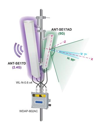
As the ANT-SE17D/ANT-SE17AD can effectively enhance the performance and coverage of the 802.11ac 2.4/5GHz environment, it is also quite suitable for outdoor wireless LAN applications, such as point-to-point connection between the warehouses.
