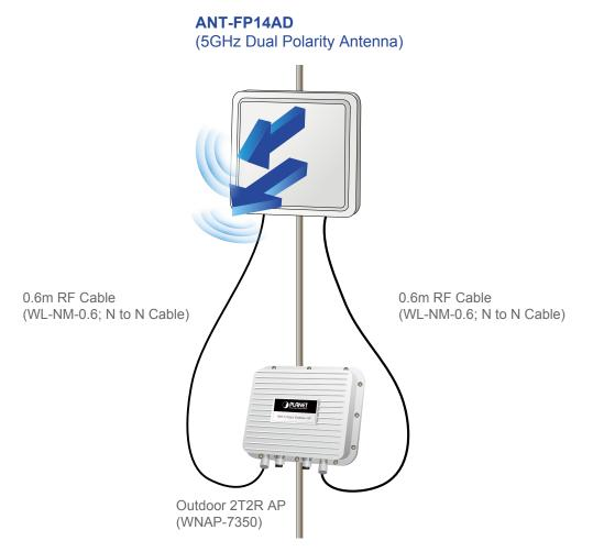
\* For extension, you can add WL-N-10 N-Male (male pin) to N-Female (female pin) between RF Cable and Antenna.
