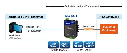
The advantage of having the IMG-120T is to assist users to build an industrial environment between the Modbus TCP/IP Protocol and the Modbus RTU/ASCII Protocol easily, thus offering an application solution to the industrial control equipment without Ethernet ports. Thus, the industrial control equipment can only control through an industrial PC workstation or industrial control panel.
