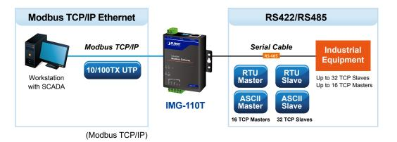
The advantage of having the IMG-110T is to assist users to build an industrial environment between the Modbus TCP/IP Protocol and the Modbus RTU/ ASCII Protocol easily, thus offering an application solution to the industrial control equipment without Ethernet ports and the industrial control equipment can only control through an industrial PC workstation or industrial control panel.
