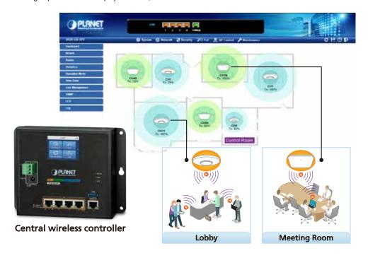
For example, to configure multiple Smart APs of the same model, the WGR-500-4PV allows clustering them to a managed group for unified management. According to requirements, wireless APs can be flexibly expanded or removed from a wireless AP group at any time. The AP cluster benefits bulk provision and bulk firmware upgrade through single entry point instead of having to configure settings in each of them separately.
