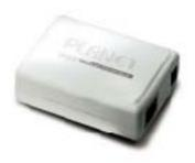
For the cost saving and power management purpose, PLANET releases a new 10/100/1000Mbps Power over Ethernet Injector POE-152.
