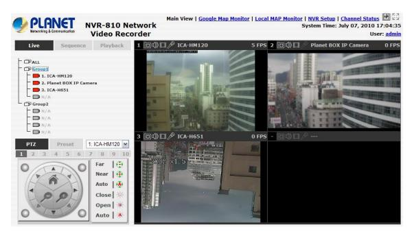
The 8 channel NVR comes with a 8-video split window view with one video displays on a larger window. Select a channel from the drop-down menu to display its video on the larger split window. You can also double-click on any of the smaller one to display its video to the larger window.
