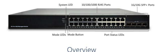
PSGS-2628XL L2+ Managed PoE+ Switch is a next-generation Ethernet Switch offering full suite of L2 features, additional 10GbE uplink connections, better PoE functionality and usability, including advanced L3 features such as Static Route that delivers better cost performance and lower *total cost of ownership* in Enterprise networks via fiber or copper connections.
